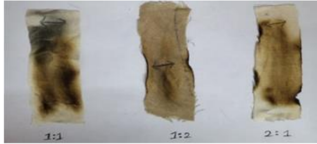
Figure. 4.3.1: Flammability test of MEPPE + TiO 2 NPs finished cotton fabrics
