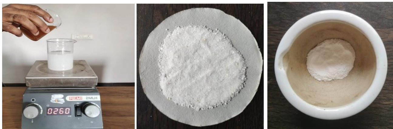
Figure 3.6.1 TiO 2 nanoparticle synthesis and converting into powder form
