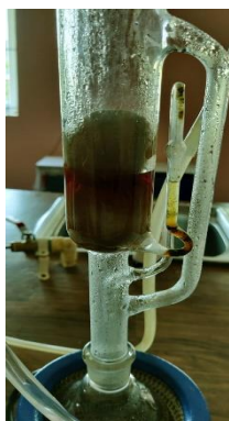
Soxhlet extractor and extraction process
